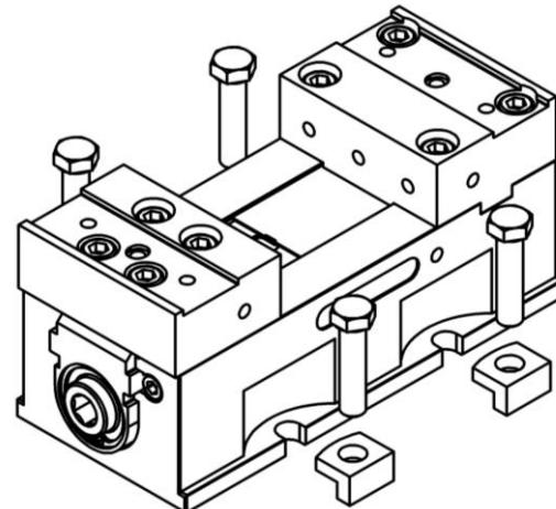
In its basic version, the KSO has 4 x Ø12 H7 positioning holes with which to position it on grid plates with a grid of 50 and in T-slot tables. The KSO is fixed from above using 4 No. M12 x 50 cylinder screws and 4 clamping claws.
